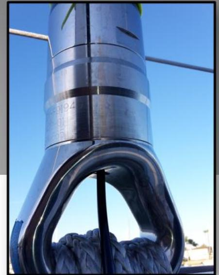
The ILSense is inserted between the tapped end of the cable and the thread of the end fitting.
